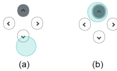
Figure 5.6: Manual gaze calibration shifts users can use before starting the application to change the gaze offset. (a) Shows the initial offset and (b) shows the gaze point after manual calibration.
