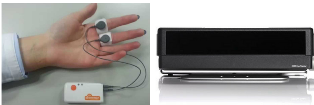
Figure 3.5: Left: Shimmer Galvanic Skin Response (GSR) device. Right: Tobii X60 Eye Tracker.
