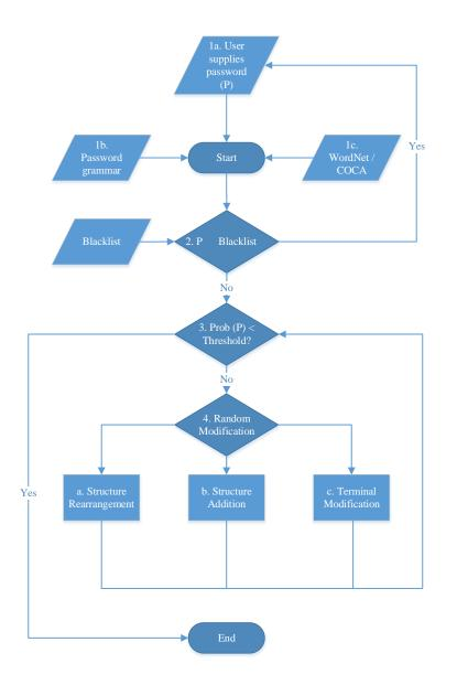
Fig. 4.2 Flowchart describing the PassMod strengthening algorithm.
